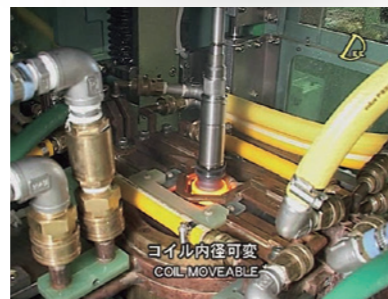
The coils are formed by pinching from upper and lower side in a similar motion to folding a laptop computer.
