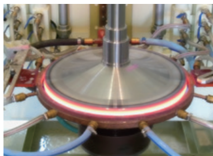
The photo shows the hardening of the trolley for a gantry crane (outer diameter 500mm, height 100mm).
