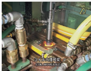
The coils on the upper side can be moved. The coils are formed by pinching from upper and lower side in a similar motion to folding a laptop computer.
