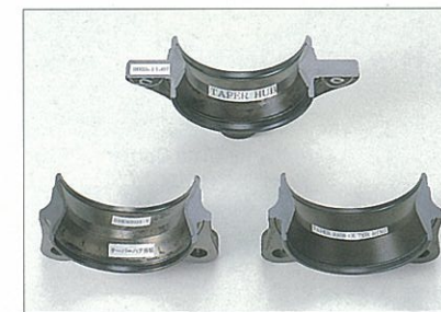
Hardened layer for Hub Unit Outer ring HUB UNIT 外輪 焼入硬化層
