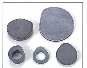
Hardened layers of various camshaft 各種カムシャフト焼入硬化層
