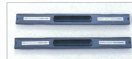
Hardened depth for Dual Frequency Combined Heat-treating Drive shaft 2周波合成ドライブシャフト焼入硬化層
