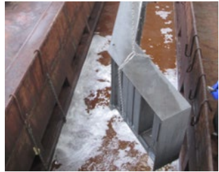
Rust-removal process (degreasing, pickling, etc.)
