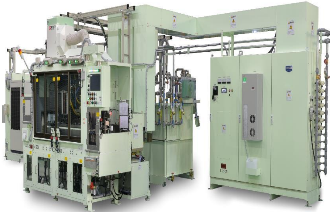
Hardening and tempering equipment for EV motor shafts
